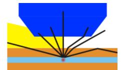
Principle of immersion microscopy. Path of rays with immersion medium (vellow) (left half) and without (right half). Rays (black) coming from the object (red) at a certain angle and going through the cover-slip (orange, as is the slide at the bottom) can enter the objective (dark blue) only when immersion is used. Otherwise, the refraction at the cover-slip-air interface causes the ray to miss the objective and its information is lost.
